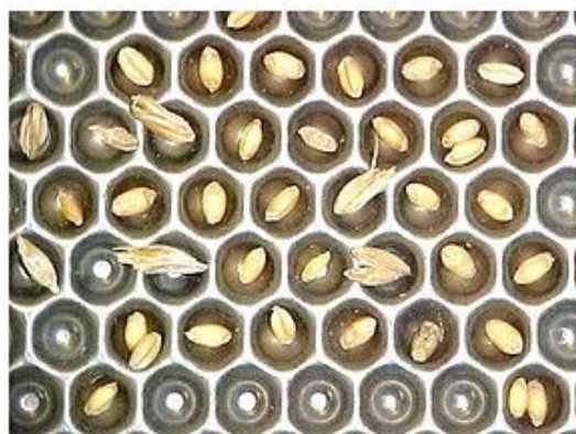
Interior of Indented Cylinder
